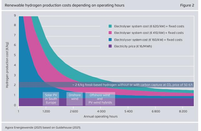
The figures are estimates for illustrative purposes and are based on full-load hours that can be reached with renewable energy sources across Europe. The transparent boxes show the full-load hours of corresponding renewable energy sources.
