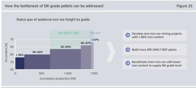
Agora Industry and Wuppertal Institute (2023), based on MPP (2021). Note: DRI-SMELT-BOF = direct reduced iron – electric smelter – basic oxygen furnace; DRI-EAF = direct reduced iron – electric arc furnace. DR-grade pellets refers to direct reduction grade pellets, which are required for the DRI-EAF route, but not the DRI-SMELT-BOF route.
