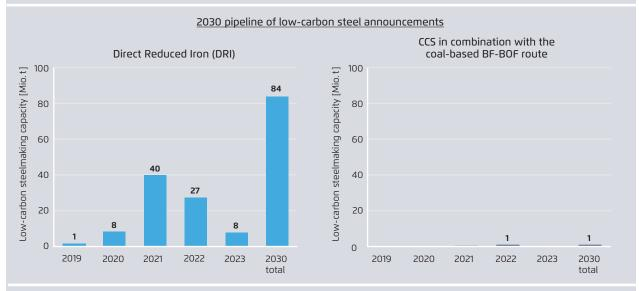
Agora Industry, Global Steel Transformation Tracker (2023). Note: The 2030 project pipeline of DRI plants includes  $H_2$ -ready DRI plants that may operate with natural gas initially. To date, the 3D project in Dunkirk is the only demonstration-scale CCS project on the BF-BOF route announced and aims to capture 1 MtCO<sub>2</sub> per year.
