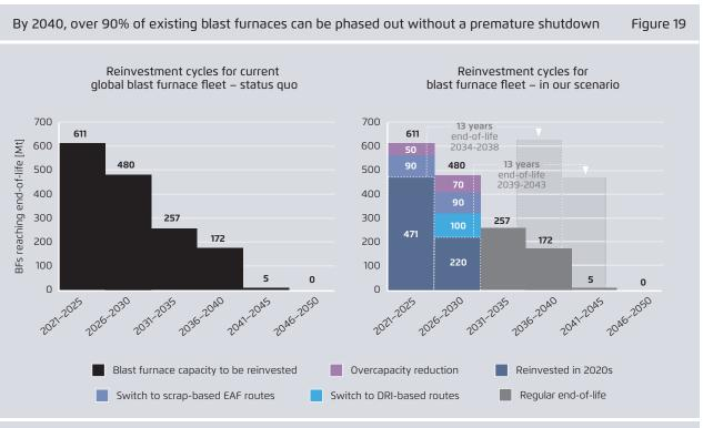
Agora Industry (2023), authors' calculations based on Global Steel Transformation Tracker (2023). Note: We assume that out of 150 Mt additional DRI capacity that could be built by 2030, 100 Mt are used to replace existing capacity. Overcapacity reduction assumptions are based on company announcements and an estimation of the capacity swap mechanism in China.
