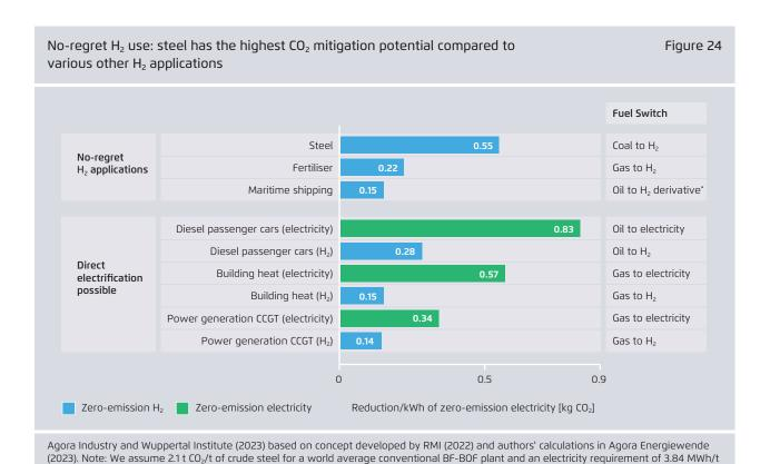
of crude steel for the DRI-EAF route that runs on 100% renewable  $H_2$ . For maritime shipping based on RMI 2022, we assumed that ammonia replaces heavy fuel oil in a 39% efficient internal combustion engine. All other assumptions are retrieved from Agora Energiewende (2023).
