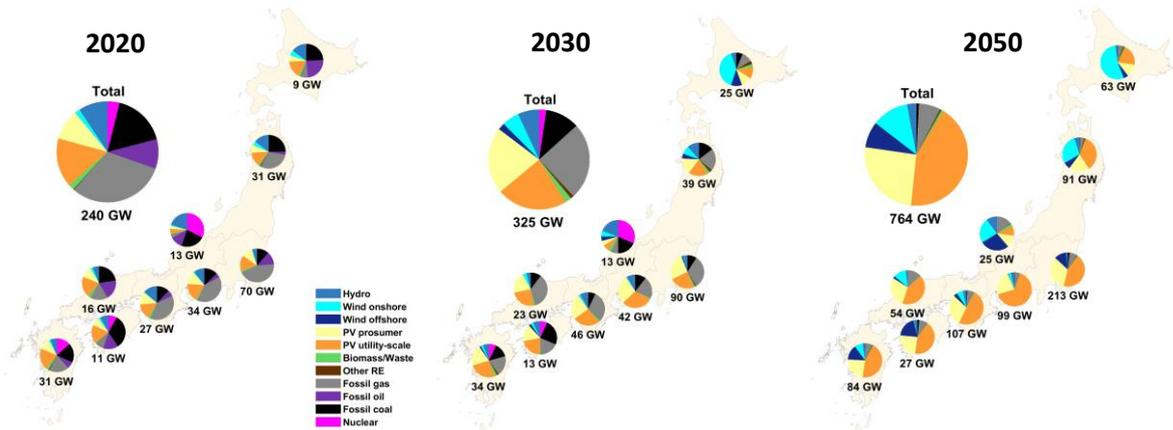
Figure 4.5: BPS all import – regional electricity generation capacities in 2020 (left), 2030 (center), and 2050 (right).
