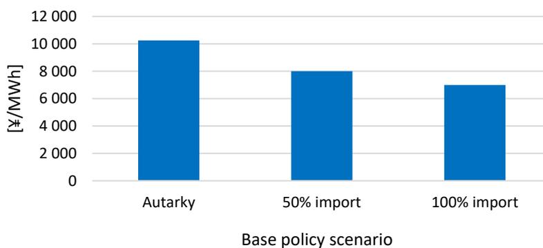
Figure 4.19: Levelized cost of heat in the Base Policy Scenario in various energy dependency settings.
